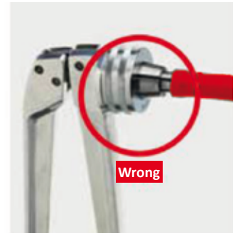
Tube not correctly plugged on the expander head
