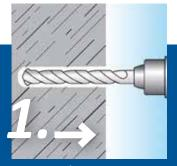
drill hole (Ø 12 mm for M8, Ø 14 mm for M10)
